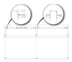
**8.** Install the fabric support profiles with the fabric preinstalled on to the rafters. The fabric support profiles go rafter by rafter onto the carriers. They slide over the thread on the bottom of the carriers in place with the nuts. While installing the fabric, you must fasten the nuts simultaneously on the fabric support profiles.
