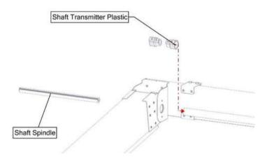
**6**. Place a shaft spindle through the rail and insert the shaft transmitter plastic on the spindle to connect to the other spindle.
