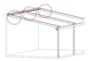
**3.** Place a hexagonal shaft spindle into the transmission tube.
