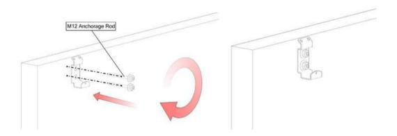
**3.** Install the wall profile on the wall mounting brackets.
