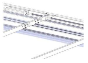
2. OPTIONAL: You can install the optional LED control box to the cross beam.
