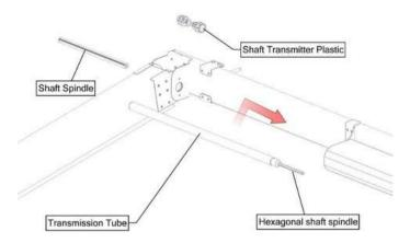
**5.** Insert a shaft transmitter plastic on to the transmission tube on the inside of the system.
