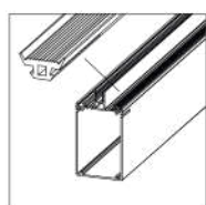
11. Side beam 1x sealing rubber
