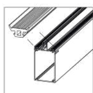
12. in between beam 2x sealing rubber
