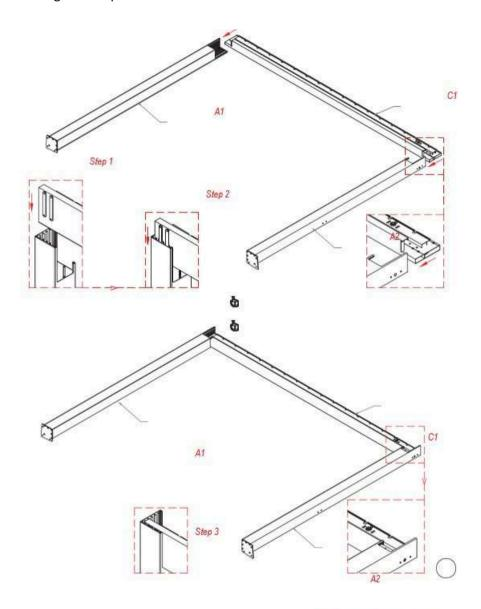
**4.** Make sure the bolts are fully tightened.
