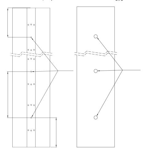
c. Drilling the holes: Remove the drilling jig and drill the pre-drilled holes through with a drill of Ø10 mm.
