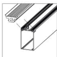
12. in between beam 2x sealing rubber
